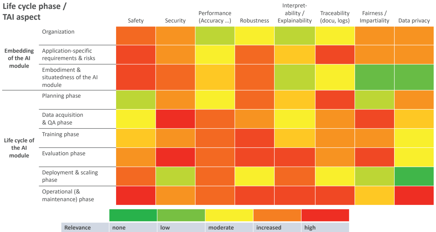
Figure 54: Relevancies of the combinations for the use case evasive manoeuvres (Source: Arndt von Twickel, Martin F. Köhler)
