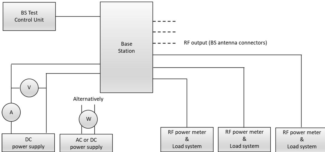
NOTE: BS as defined in Figure 1 (integrated BS) or Figure 2 (distributed BS). AC supply to be used for BS with build in AC power supply, otherwise default DC supply voltage as specified in clause 5.2.
