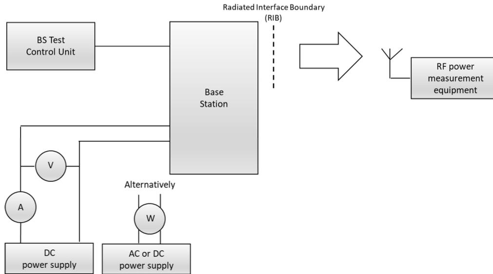
NOTE: BS as defined in Figure 2 (distributed BS). AC supply to be used for BS with built in AC power supply, otherwise default DC supply voltage as specified in clause 5.2.
